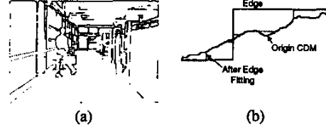
Fig. 2. Results of (a) morphological edge detection operation and (b) morphological edge fitting operation.
